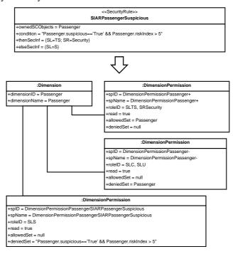
Figure 10: Logical Model: SIAR passenger suspicious
