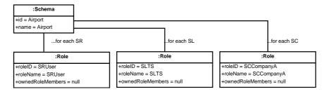
Figure 6: Logical Model: Security Configuration
