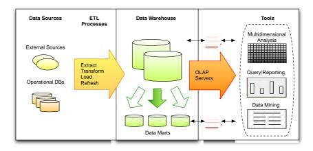
Figure 1: A Data Warehouse Architecture
